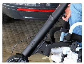
4. Lift the F35 and insert docking pins into hook on central bracket.
