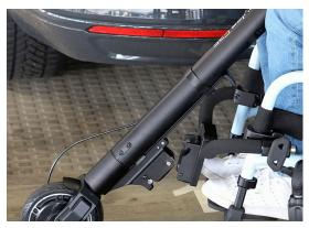
3. Line up the docking pins to the hook in the central bracket.
