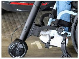
Push the handlebar forwards/ upwards until the locking mechanism clicks into place.
