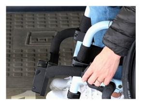
2. Secure the clips on both sides and wind the handscrews hand tight.
