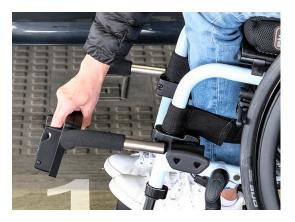
1. Line up subframe to clamps and insert all the way up to padding.
