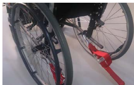
Fitting the Rear Restraint
