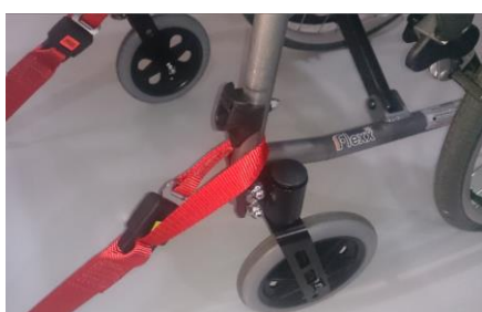
Fitting the Front Restraint
