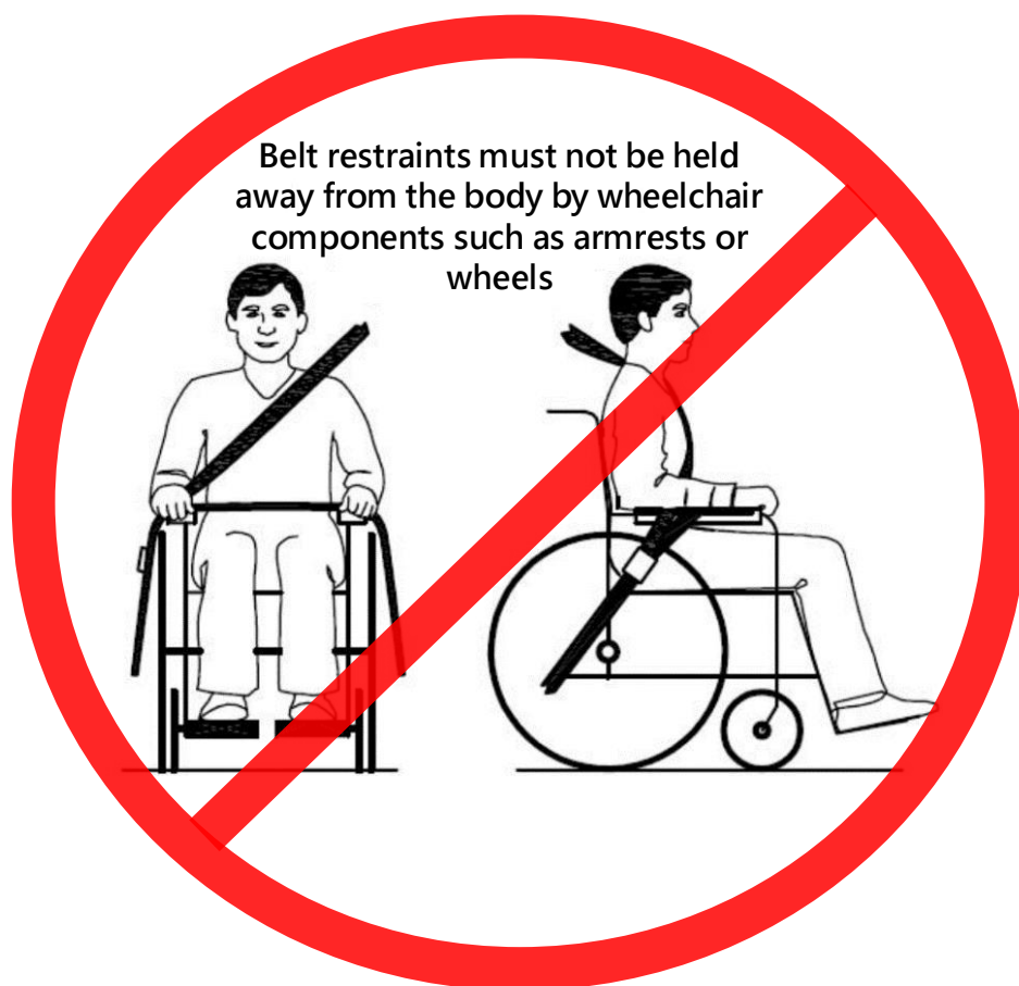
Illustration of improper belt-restraint fit
