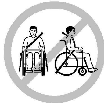
Incorrect seat belt position
