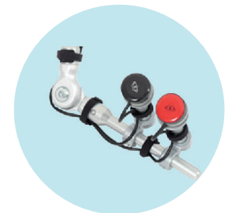
Variant multi functional switch: EU143 Piko button
