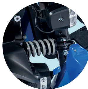
EF001 Swing arm suspension
